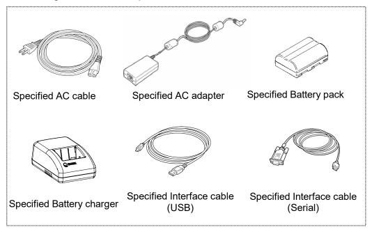
The AC adapter and the battery charger is not bundled with an AC cable. Be sure to purchase our specified options. Refer to 11 SPECIFICATIONS for using the options in the countries which have complied with regulations.
