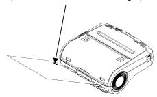
(5) To discharge the thermal paper from the printer, hold down the FEED switch.
