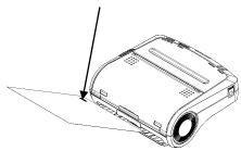
(5) To discharge the thermal paper from the printer, hold down the FEED switch.
