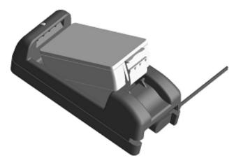
Figure 19-5 Installing Battery Pack (1)
