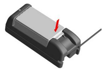
Figure 19-6 Installing Battery Pack (2)
