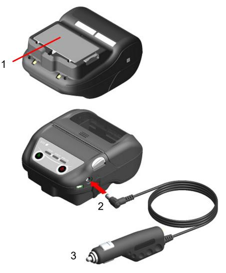
Figure 18-3 Charging in Power Off Charging Mode by Car Charger
