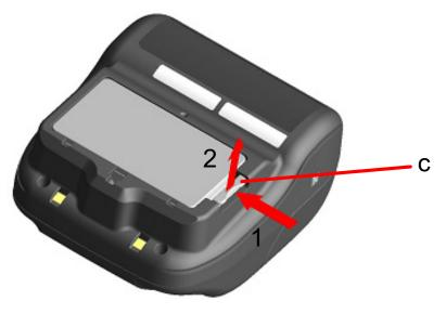
Figure 8-4 Removing Battery Pack
