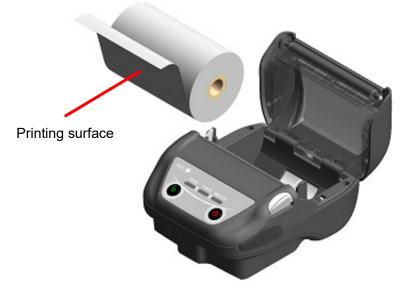
Figure 9-2 Thermal Paper Setting Direction
