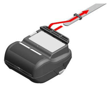
Figure 15-7 Installing Shoulder Strap (3)
