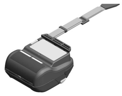
Figure 15-8 Installing Shoulder Strap (4)
