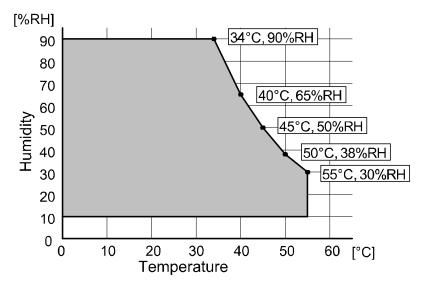
Figure 22-1 Operating Temperature and Humidity Range (Printing)
