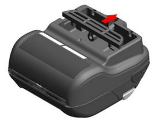
Figure 15-5 Installing Shoulder Strap (1)
