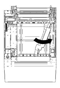
(5) Put the hook which is located on the upper side of the partition plate R or partition plate L on the hole of paper holder as shown in the figure below.
