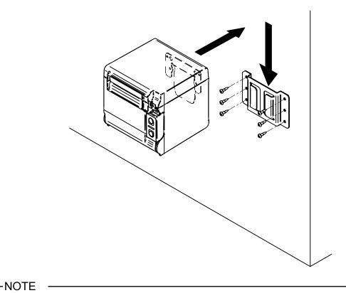
Check the place and the material/structure of the wall, and then install the printer securely. Injury or destruction of property might occur by dropping off.
