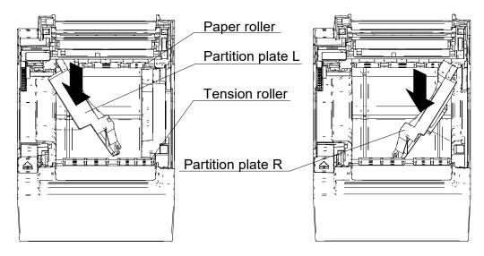
(4) Rotate the partition plate R or partition plate L within the paper holder in the direction of the arrow shown in the figure below to make the side surface of the paper holder and the partition plate in parallel.
