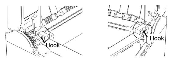
(6) Push the partition plate R or partition plate L to the direction of the arrow shown in the figure below with placing them along the side surface of the paper holder, and then put the projection which is located at the bottom of the partition plate in the hole of the paper holder.
