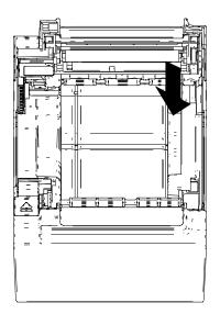
(7) Turn the printer over, and make sure that the projection of the partition plate R or partition plate L is fit properly into the hole of the paper holder (the arrow shown in the figure below).
