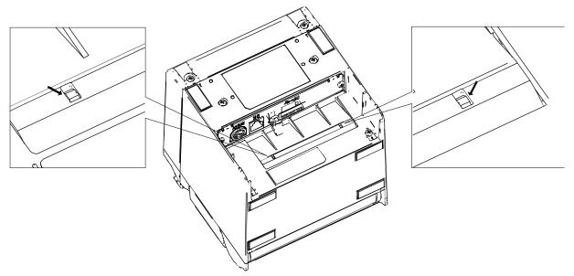
See "RP-D10 SERIES THERMAL PRINTER TECHNICAL REFERENCE" to set the MS4-4 (Paper Width Selection) to 58 mm.
